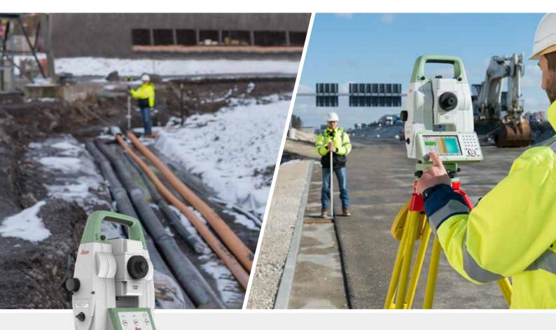
Sometimes you need your instrument to grow with your projects. The Leica TS13 empowers you to start with two-person mode and upgrade the instrument gradually to a robotic total station. You decide when to upgrade it – you can choose a different **keyboard**, add **lock** to follow a moving target or include **robotic capabilities** with **SpeedSearch** and controller **connectivity** via a radio handle. The TS13 comes with **AutoHeight**, helping you to setup your instrument error-free.
